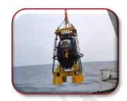
➤ 'MATSYA 6000' vehicle is being designed and developed by National Institute of Ocean Technology (NIOT), Chennai under Ministry of Earth Sciences. It has an endurance of 12 hours under normal operation and 96 hours in case of emergency for human safety.
