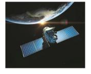
GAGAN has been jointly developed by the Indian Space Research Organisation (ISRO) and the Airports Authority of India (AAI). By using uplink and reference stations, this system provides corrections to the global positioning system (GPS) signal so as to improve the management of air traffic.
