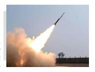
All of the **mission's goals were met throughout the test.** The missile's SFDR-based propulsion can intercept aerial threats at supersonic speeds over extended distances. It has an estimated range of 350 kilometers, which is exceptionally long.
